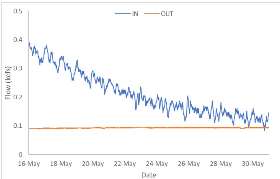
**Figure 43. Hourly Flows Inflow vs. Outflow (RO) (Fall Creek Tailrace)**
