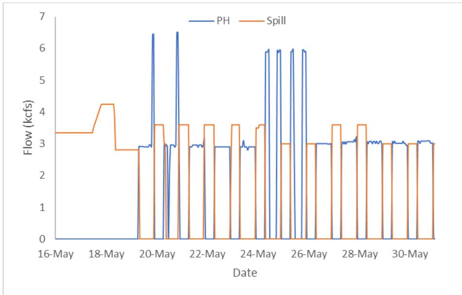
**Figure 59. Hourly Flows PWR vs. Spill (Lookout Dam Tailrace)**
