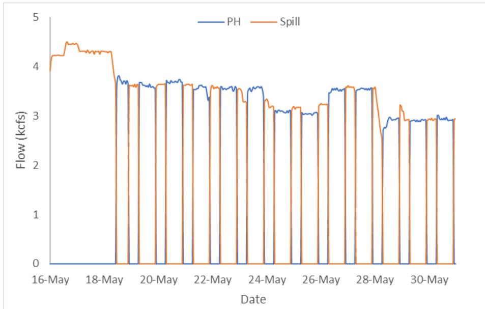
**Figure 53. Hourly Flows PWR vs. Spill (Dexter Dam)**
