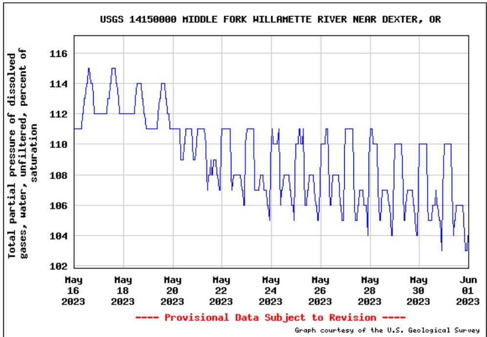
**Figure 51. Total Dissolved Gas Saturation (%); Middle Fork Willamette River, Near Dexter, OR**
